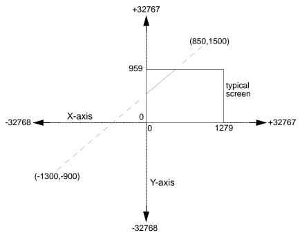
Note: Many of the graphics examples in this and the following chapters start with the command MODE MODE. This performs a mode change to the mode you are currently in, resetting the state of the VDU drivers and clearing the screen, but leaving the resolution and number of colours unchanged.
